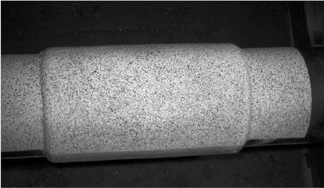
Figure 3: Pipe spool survival specimen with stochastic speckle pattern applied for DIC imaging
