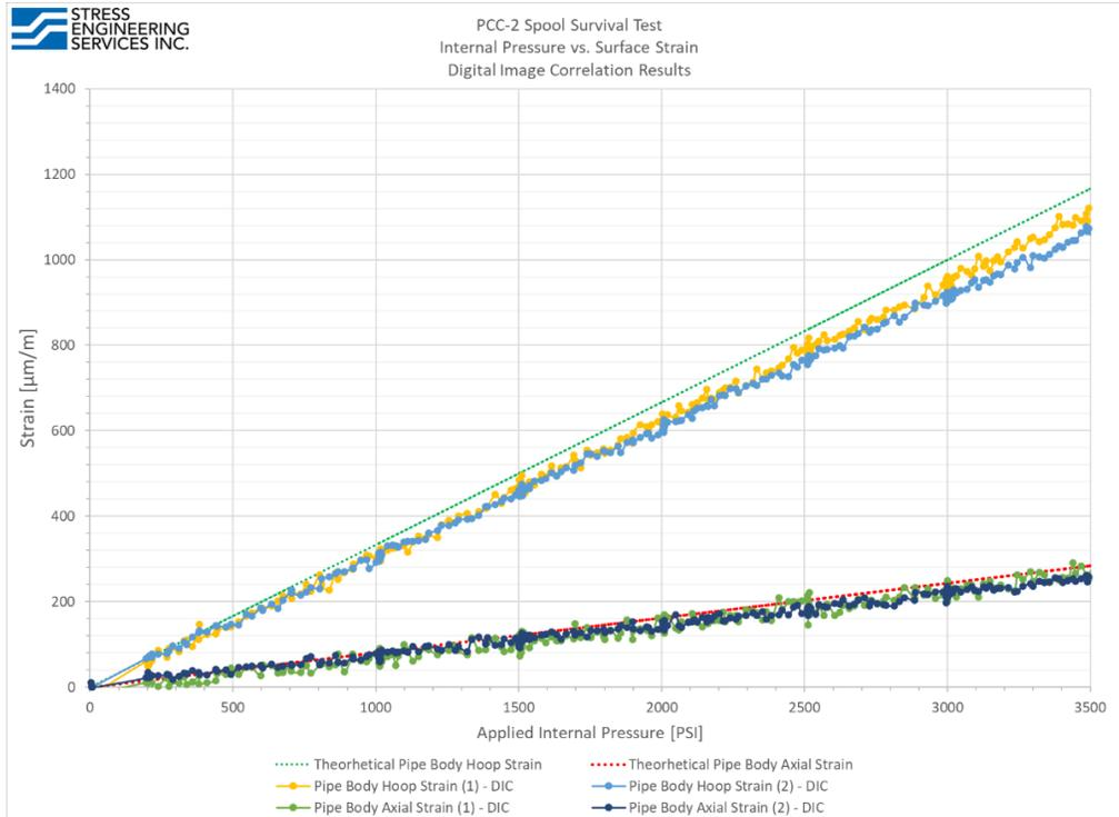
Figure 8: Plot of pipe body strains acquired using DIC and theoretical pipe body strains vs. internal pressure
