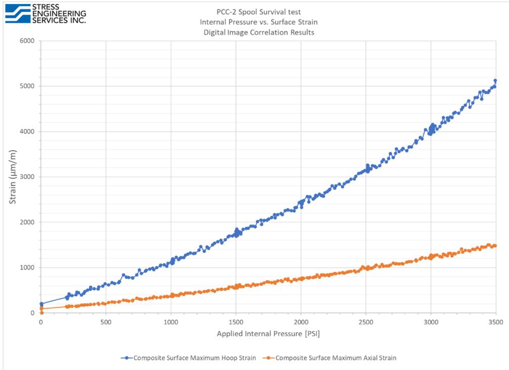
Figure 9: Plot of recorded composite repair strains acquired using DIC vs. internal pressure
