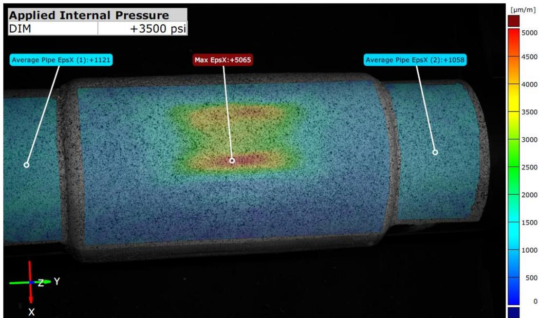
Figure 6: Overlay of composite repair and pipe body hoop strain at 3,500 PSI acquired using DIC during pipe spool survival pressure test.
