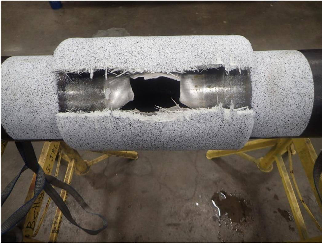
Figure 5: Photograph of sample following spool survival and burst test, illustrating failure in machined wall loss region
