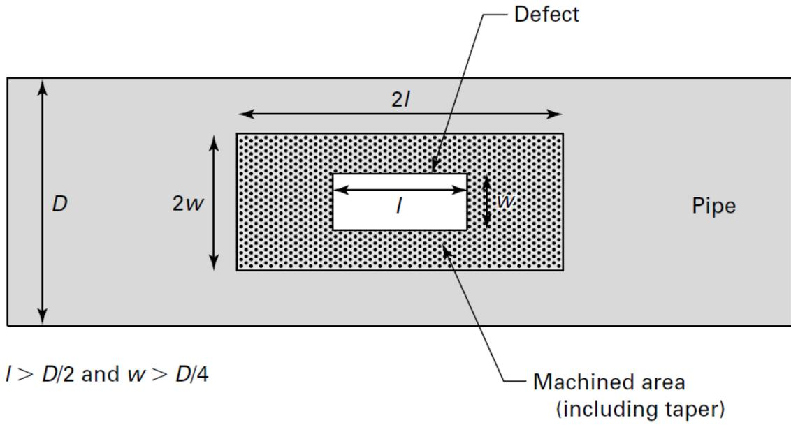
*Figure 1: ASME PCC-2 pipe spool survival specimen specifications*
